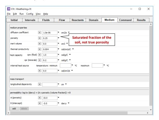
we set up our model to be 25% saturated. "Porosity" in the model represents the saturated fraction of the soil, rather than the true porosity, which includes the unsaturated fraction. The flow velocity, as we calculate from the discharge and saturated soil fraction (i.e.  $v = q/\phi$ ), is 16 m/yr.
