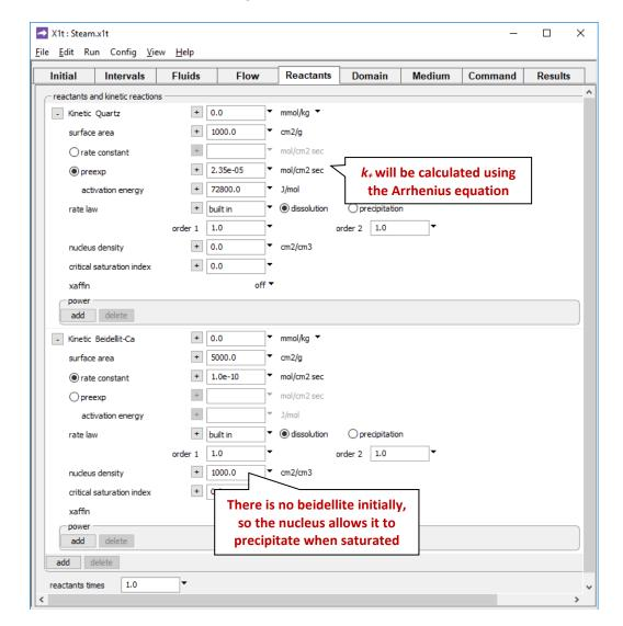
On the **Reactants** pane, we assign rate laws for quartz and calcium beidellite.
