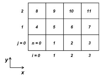
In general, columns of nodes are indexed i = 0 to  $N_x - 1$ , and rows from j = 0 to  $N_y - 1$ . The index n of a node at column i and row j is given by the equation
