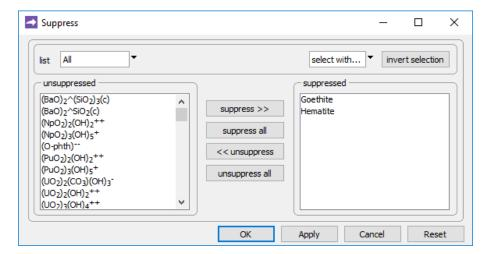
we suppress the most stable ferric minerals, to allow the iron to remain in ferric hydroxide form.
