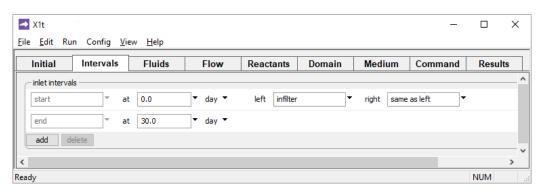
time span in the model is set to 30 days.
