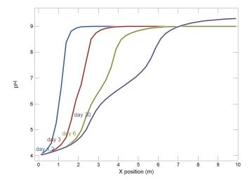
After about 20 days, the pH profile across the domain converges to a steady state in which supply of  $H^+$  by the infiltrating water and consumption of acid by calcite dissolution fall into balance.
