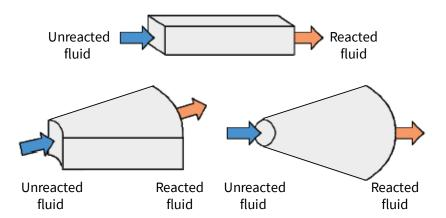
The flow of fluid along the domain displaces reacted fluid from the opposite end.
