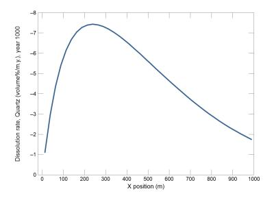
In making this plot in **Xtplot**, we select **Plot** → **XY Plot...**, then on the **Y Axis** tab, next to "Variable type", select "Reactant properties", then "Dissolution rate, Quartz".
