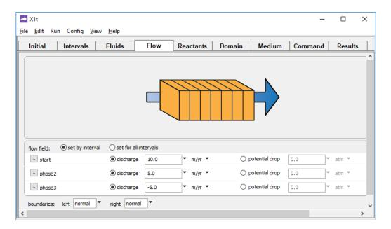
In the latter example, flow slows, then changes direction as the simulation proceeds.
