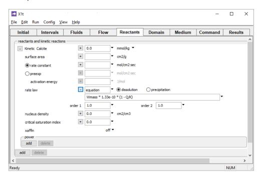
we define a simple kinetic rate law that describes dissolution of calcite into the infiltering water, as a function of water mass and the mineral's saturation Q/K.
