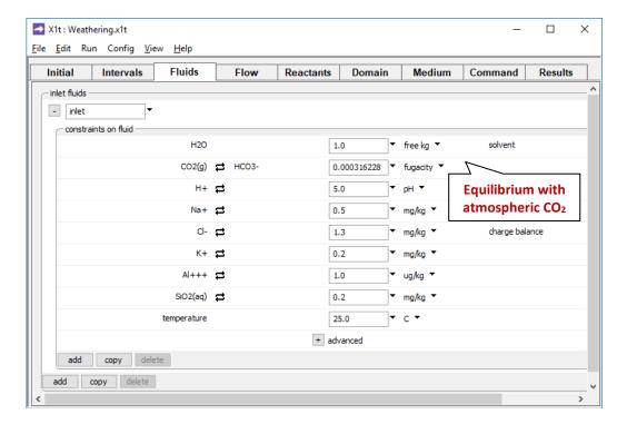
we set the inlet fluid in the simulation to be dilute water in equilibrium with atmospheric CO<sub>2</sub>.
