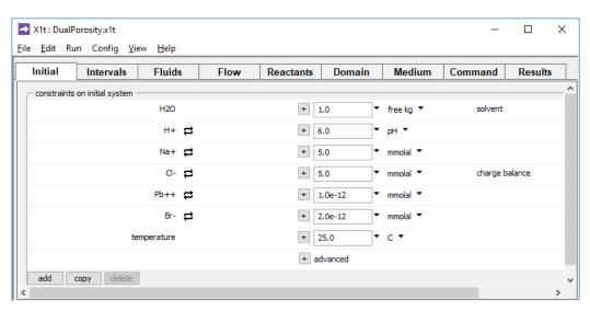
the initial fluid is a NaCl solution of pH 6 containing almost no Pb++.
