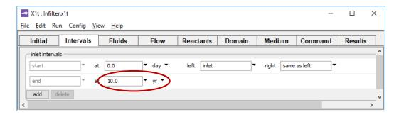
This change has the effect of prescribing a faster groundwater flow rate of 1000 m/yr, since the pore fluid will still be displaced 100 times.
