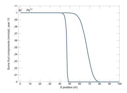
On the **Y Axis** pane, change the "Display" pulldown to "One value at several times" and select Pb++, then change the scale to "log". Select multiple steps on the **Time Level** pane. Plotting the Pb composition of the fluid on a log scale versus X position over the course of the simulation, we see that after 40 years of flushing with fresh water, Pb concentration remains well in excess of the drinking water standard of 15  $\mu$ g/kg.
