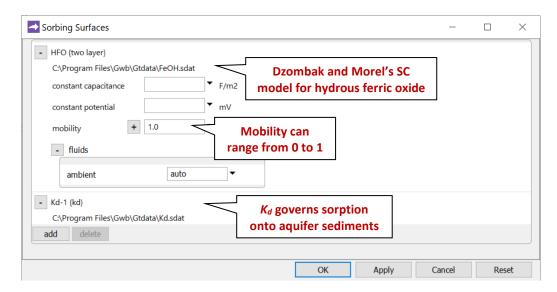
The former supplies a distribution coefficient  $K_d$  governing sorption of Pb<sup>++</sup> onto the aquifer sediments. The latter contains Dzombak and Morel's (1990) compilation of surface complexation reactions for hydrous ferric oxide.
