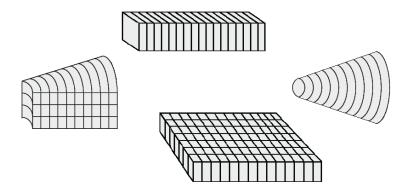
In the examples above, the nodes are spaced evenly. In other words, the dimensions  $\Delta x$ ,  $\Delta y$ ,  $\Delta z$  (or  $\Delta r$ ,  $\Delta \theta$ ,  $\Delta y$ ) of each block are the same.
