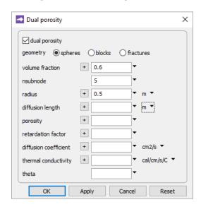
sets a dual porosity model in which the stagnant zones are composed of spheres 1 m across; the spheres take up 60% of the domain's volume. You must, at a minimum, set values for  $X_{\text{stag}}$  and  $\delta$ ; as field variables, these values can vary across the domain.
