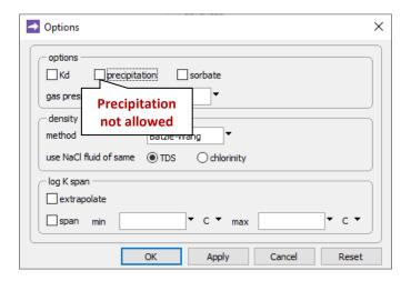
the precipitation option has been deselected. As a result, the only minerals that can precipitate are those already in the system and those for which a kinetic rate law has been set.
