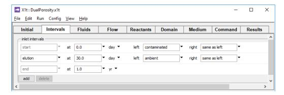
we set an **X1t** simulation composed of two intervals, the first spanning 1 month, and the second extending from that time to 1 year.
