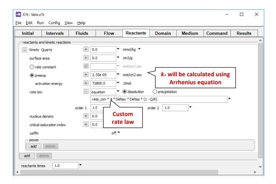
Here, we set a nominal value for specific surface area, as required by the program, although we do not use this variable.
