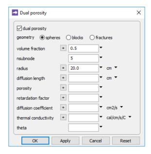
The stagnant zones in the model are composed of spheres 40 cm across that make up half the aquifer's volume.
