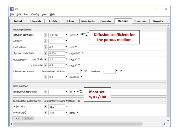
or with the diffusion\_coef and dispersivity commands. By default, the program assumes that  $D^*$  is  $10^{-6}$  cm<sup>2</sup>/s and  $\alpha$  is the length of the domain L divided by 100.
