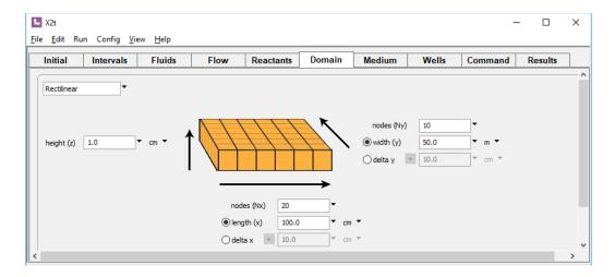
or with the length, width, Nx, and Ny commands. The settings above define a 100 m × 50 m domain composed of 200 nodal blocks, each of which is 5 m × 5 m (i.e.,  $\Delta x$  and  $\Delta y$  are both 5 m).
