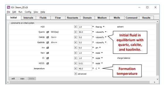
we set the formation temperature to 40°C and define the formation mineralogy and pore fluid composition as we did in the **X1t** example. The simulation will span 20 days.
