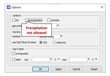
we unset the precipitation option. By doing so, we prevent other minerals, such as cristobalite and amorphous silica, from forming, although, of course, we could generalize the simulation to account for the various silica polymorphs.
