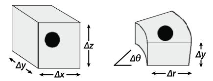
Each nodal block has fixed dimensions  $\Delta x$ ,  $\Delta y$ , and  $\Delta z$  in a linear domain,  $\Delta r$ ,  $\Delta \theta$ , and  $\Delta y$  in a radial domain, or  $\Delta r$  and  $\Delta \theta$  in a spherical domain. A nodal point is located at the center of each block, as shown.
