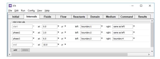
sets three reaction intervals—"start", "phase2", and "phase3"—beginning at 0 years, 2 years, and 6 years, during which the fluids "boundary1", "boundary2", "boundary3", and "boundary4" lie along the domain boundaries; the simulation in the example continues to 10 years.
