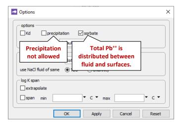
the precipitation option has been deselected. This setting prevents stable but slow-forming ferric minerals like goethite (FeOOH) from appearing in the simulation, at the expense of the  $Fe(OH)_3$  precipitate.
