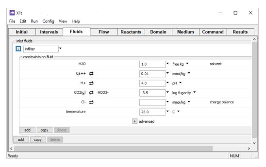
defines a water "infilter" that is more acidic and dilute than the initial fluid, and is in equilibrium with atmospheric  $CO_2$ .
