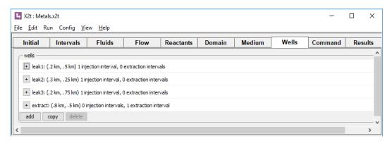
The first three slowly leak the contamination fluid into the aquifer over the first 10 years. The remaining well, at the bottom of the list, is the remediation well. It withdraws water from the aquifer, so the injection rate is set to a negative value.
