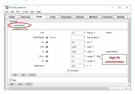
we set the contaminated fluid to a dilute water in equilibrium with ferric hydroxide [Fe(OH)<sub>3</sub>, a proxy for hydrous ferric oxide], containing 0.1 mmolal inorganic Pb (about
