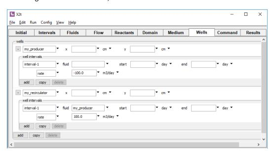
the well "my\_recirculator" injects water extracted from the domain by well "my\_producer". The commands
