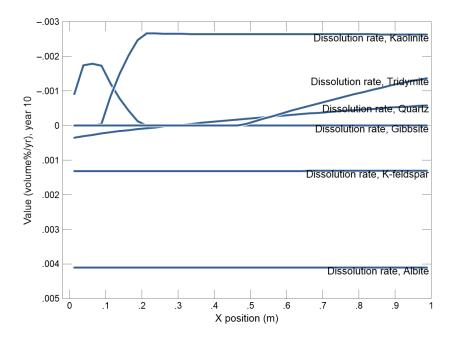
According to this diagram, K-feldspar and albite dissolve throughout the profile, in response in part to  $CO_2$  supplied by the soil gas. Near the top of the profile, quartz dissolves as well, and gibbsite and kaolinite precipitate. Deep in the profile, kaolinite, tridymite, and quartz precipitate.
