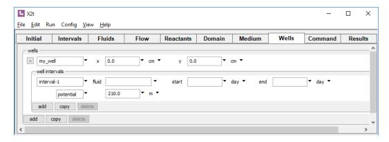
defines the water level in "my\_well". If the head in the neighboring nodes is higher than this value, the well will produce water; if lower, water will flow into the domain. You can set the head in units of mm, cm, m, km, in, ft, or mi, and hydraulic potential as Pa, Mpa, atm, bar, or psi. The command
