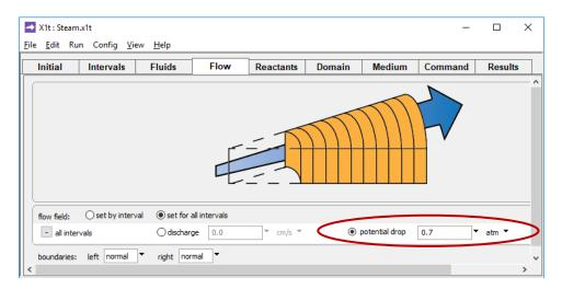
we assume an injection pressure 0.7 atm greater than the formation pressure to provide a drive for flow.
