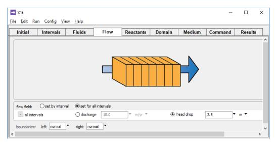
In the latter case, the program calculates the flow field from the head drop, the permeability field, and the fluid's viscosity.
