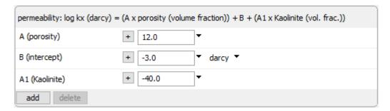
By this correlation, permeability increases with increasing porosity, but the presence of kaolinite serves to decrease the permeability, as shown below:
