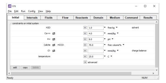
Here we see that calcite makes up 70% of the initial system's volume, leaving a porosity of 30%, and that equilibrium with the mineral constrains bicarbonate concentration. The pH is set to 9 and the initial fluid contains 4 mmol/kg Ca<sup>++</sup>, as well as chloride to balance charge.
