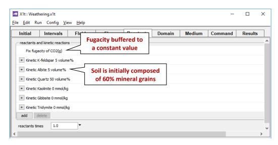
we cause its fugacity over the simulation to be buffered to a constant value.
