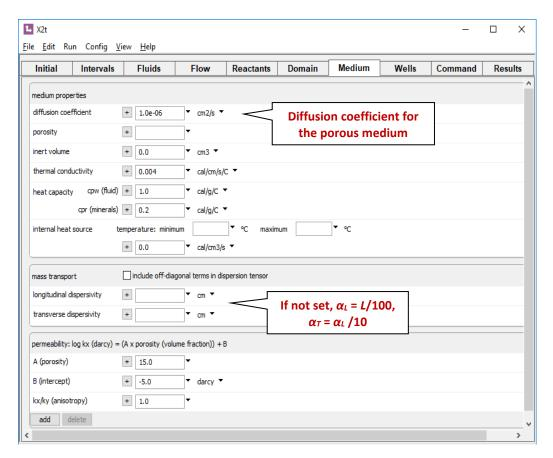
or with the diffusion\_coeff and dispersivity commands. By default, the program assumes that  $D^*$  is  $10^{-6}$  cm<sup>2</sup>/s,  $\alpha_L$  is the length of the domain L divided by 100, and  $\alpha_T$  is one-tenth of  $\alpha_L$ .
