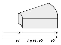
The length L of an axisymmetrical domain, then, is r1 - r2. Normally, the domain is oriented with the small-radius end to the left, but you can reverse its sense.
