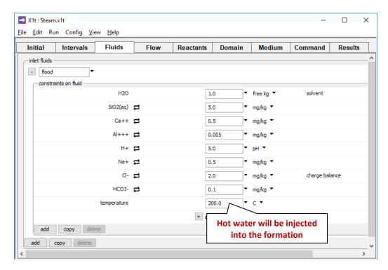
we set a boundary fluid "flood" to represent the steam (actually hot water). The fluid's composition reflects fresh water heated to 200°C.
