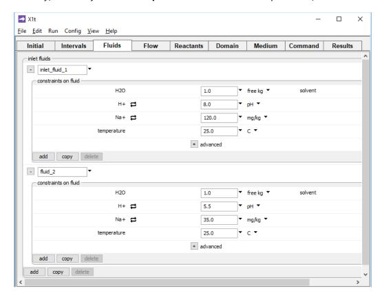
we've created two fluids, "inlet\_fluid1" and "fluid\_2", and constrained their compositions. To use the command line, enter a scope command followed by a name for the fluid, then constrain each basis entry. The commands
