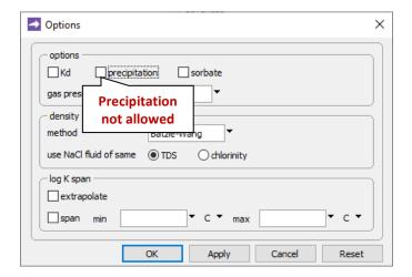
the precipitation option has been deselected. As a result, no minerals are allowed to form except for those in the initial system and those for which we set kinetic rate laws. On the **Domain** pane, we configure the model in radial coordinates.
