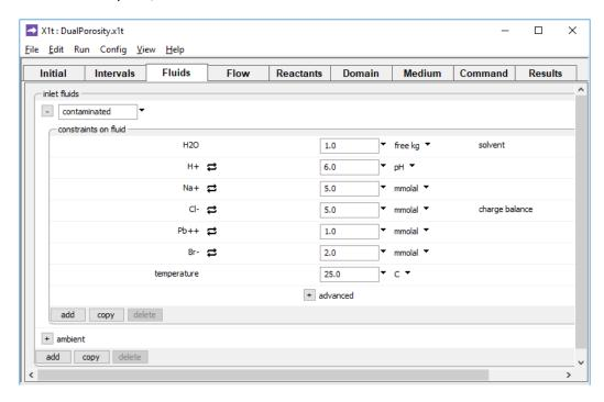
the inlet fluids for the two intervals in the simulation are the same as the initial fluid, except the fluid for the first interval contains 1 mmolal  $Pb^{++}$ , with Br as the counterion.
