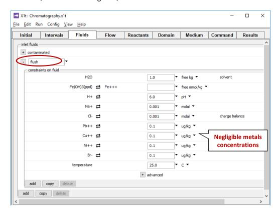
an uncontaminated water containing almost no heavy metals or bromide.
