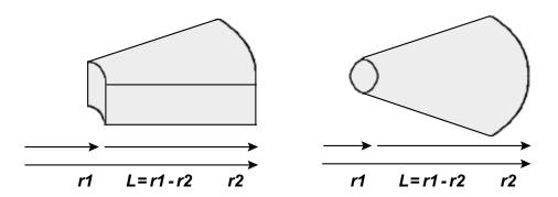
The length L of a radial or spherical domain, then, is r1 - r2.
