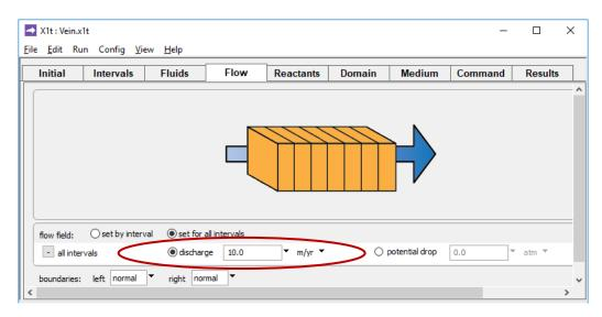
we specify an upward fluid discharge of 10 m/yr. Over the course of 1000 years, fluid in the fracture will be displaced 10 times.
