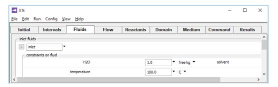
specify that a 100°C boundary fluid named "inlet" invades a domain with an initial temperature of 25°C.
