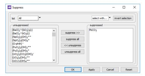
we've suppressed the PbCO<sub>3</sub> ion pair, the stability of which, in the database, is almost certainly erroneous.
