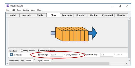
the simulation is configured to displace the pore fluid in the aquifer 100 times. Hence, the water flows at a velocity of 100 m/yr.
