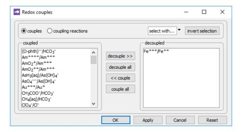
we see the redox coupling between ferric and ferrous iron has been disabled. This setting explains why we've been able to include  $Fe^{+++}$  species and minerals in the simulation, without setting basis entries representing  $Fe^{++}$  or redox state.
