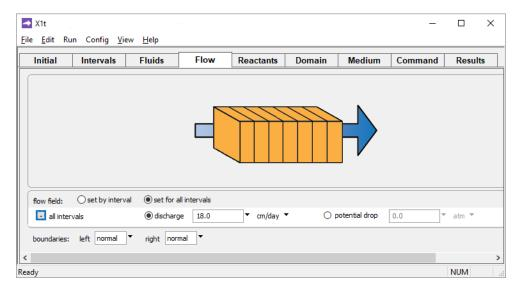
we set discharge of the infiltrating fluid into the domain to 18 cm/day. Then, on the **Reactants** pane
