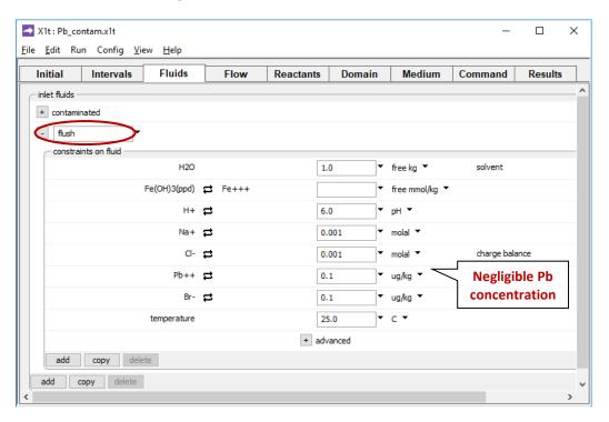
an uncontaminated water containing almost no lead or bromide.
