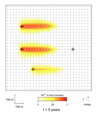
You can represent other variables on this plot using the contouring (**Format → Contour...**) and color masking (**Format → Color Mask...**) features.
