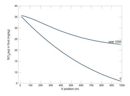
Quartz precipitates along the fracture, forming most quickly not near the surface, where it is most supersaturated, but at depth, where by the Arrhenius equation, the rate constant is largest.
