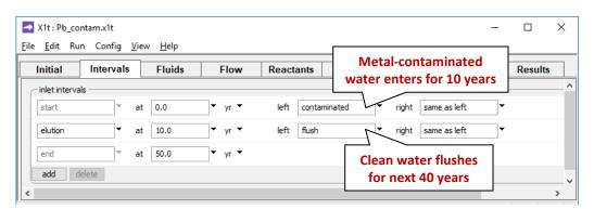
we let the simulation run over two reaction intervals for a total of 50 years. During the first 10 years, metal-bearing water contaminates the aquifer. Then, over a period of 40 years, it is flushed with clean water.
