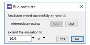
You can view the simulation results by clicking on **Plot**, or, if you have selected the "print dataset" option on the **Config → Output...** dialog, clicking on **View**. Select **No** to terminate the simulation as specified, or **Yes** to extend the simulation past the original endpoint. In the latter case, you specify a new simulation endpoint.
