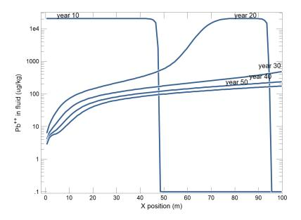
The slow decrease in Pb concentration during flushing reflects the gradual desorption of the metal from the aquifer sediment.
