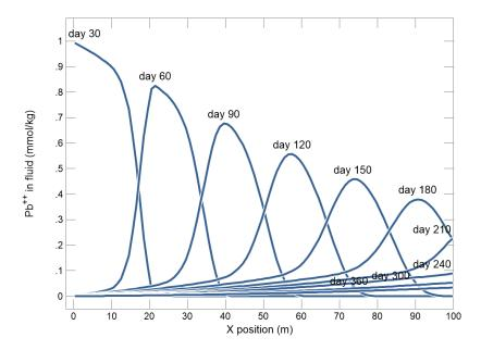
We can compare this result to the case in which the Pb<sup>++</sup> does not diffuse into the stagnant zone by setting the diffusion coefficient there to 0.
