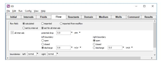
your settings apply to all the intervals in a simulation. In this example, a discharge of 0.6 m yr<sup>-1</sup> across the left boundary is applied to the left side of all of the boundary intervals in the simulation, regardless of how they might have been set by previous commands.
