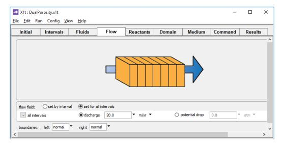
we specify that water recharges the left side of the domain at a specific discharge of 20 m/yr.
