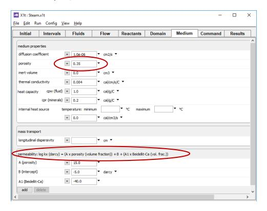
we set the initial porosity and define a correlation by which permeability varies with porosity and the volume fraction of calcium beidellite, a smectite mineral.
