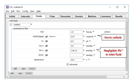
fluid passing into the domain is the same as the initial fluid, except it contains more abundant ferric precipitate, but almost no Pb<sup>++</sup>.
