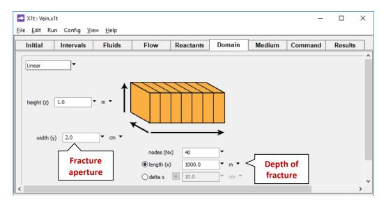
We assume the fracture extends to a depth (along x) of 1000 m and has an aperture (along y) of 2 cm. The extent of the system along z is arbitrary. We divide the medium into 40 nodal blocks.
