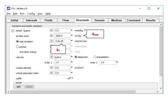
using the data of Rimstidt and Barnes (1980) and Leamnson et al. (1969). The mass of quartz carried in the simulation is the amount of buffering mineral shown in the **Initial** pane, plus the mass set in the **Reactants** pane, which here is 0.
