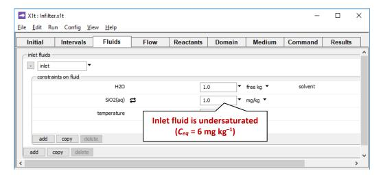
we set the inlet fluid to contain 1 mg/kg silica.
