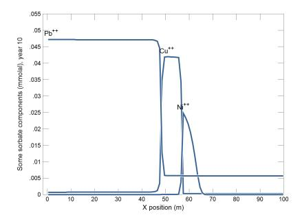
$Pb^{++}$  sorbs most strongly of the three metals, occupying the position nearest the inlet, followed by  $Cu^{++}$  and then  $Ni^{++}$ .
