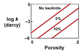
Alternatively, you can set the permeability correlation with the permeability command and arguments porosity (to set the value of A), intercept (to set B), and the names of the minerals k to be included in the correlation (to set  $A_m$ ).
