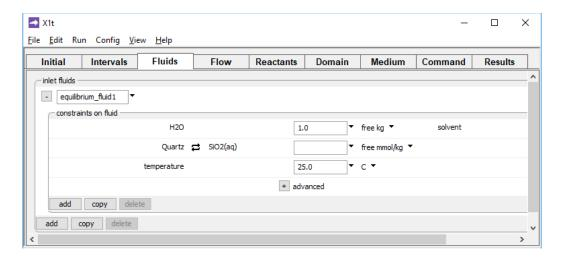
as you would when configuring **SpecE8** or **React**. In such cases, it is not necessary to set the amount of the mineral present, since the amount of a mineral in equilibrium with a fluid does not affect the fluid's composition. The following commands
