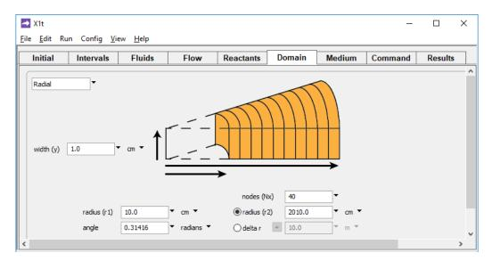
sets a domain composed of 40 nodes, starting 10 cm from the radial origin (e.g., 10 cm from the center of a well bore) and extending for 2000 cm; the radial angle is  $\pi/10$ . The default value for  $\Delta\theta$  is 0.1 radians.
