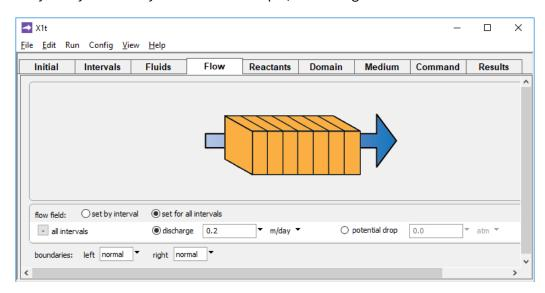
sets a specific discharge of 0.2 meters per day (or, more precisely, 0.2 m<sup>3</sup>/m<sup>2</sup>/day). The command
