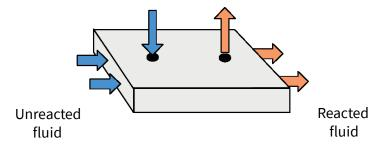
You specify whether the boundaries of the domain are open or closed to flow, and optionally the fluid discharge across them, and either the rate of flow into or out of each well, or head at the well. As with **X1t**, you set the initial conditions within the domain, as well as the composition of any fluids flowing across boundaries or injected into wells.
