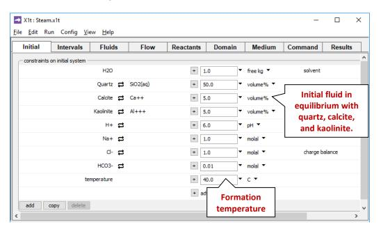
shows the conditions at the onset of the simulation. We assume that the unreacted formation contains 50% quartz, 5% calcite, and 5% kaolinite. These minerals constrain the  $SiO_2(aq)$ ,  $Ca^{++}$ , and  $Al^{+++}$  concentrations of the formation fluid. The fluid is a 1 molal NaCl solution containing a small amount of  $HCO_3^-$ ; its pH is 6. We set the initial temperature in the formation to  $40^{\circ}C$ .
