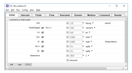
the aquifer, which includes a small amount of ferric hydroxide, contains an initially uncontaminated groundwater of the same composition as the flushing fluid.
