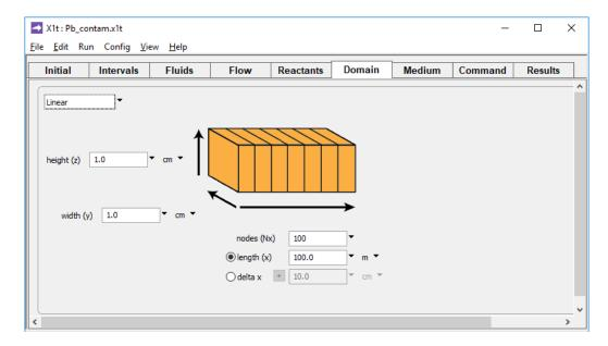
we set the length of the aquifer to 100 m and divide the domain into 100 nodal blocks. On the **Flow** pane,
