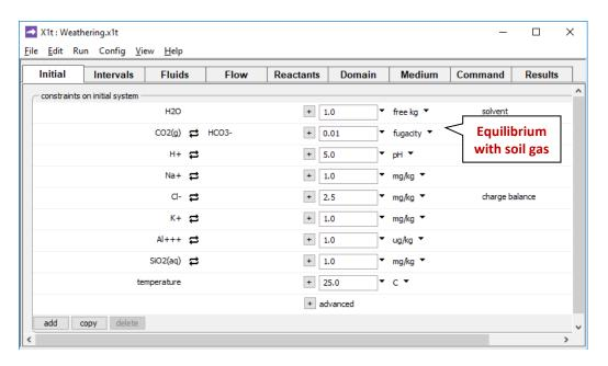
the fluid initially in the medium is also dilute, but is in equilibrium with the soil gas, which we take to have a  $CO_2$  fugacity of  $10^{-2}$ .
