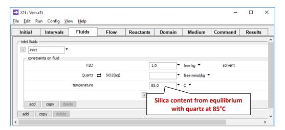
we set the silica content of the inlet fluid to equilibrium with quartz at the inlet temperature, 85°C.
