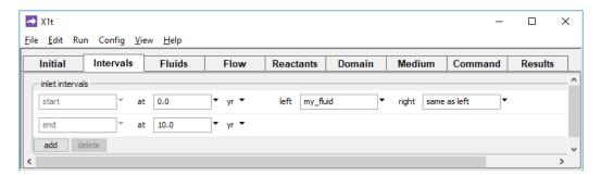
to set the beginning and ending times of the simulation, and to select the fluids to appear at the domain's boundaries.
