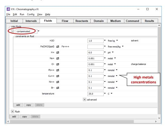
we set the contaminated fluid to a dilute water in equilibrium with ferric hydroxide  $[Fe(OH)_3$ , a proxy for hydrous ferric oxide], containing 0.1 mmolal inorganic Pb<sup>++</sup>, Cu<sup>++</sup>, and Ni<sup>++</sup>. The water also contains Br<sup>-</sup> in equal molal concentration with the metals. Since, according to the surface complexation model, Br does not sorb, it serves in our calculation as a conservative tracer.
