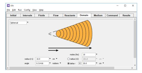
If you are working from the command line, use the spherical (or spike) command with keywords r1, r2, and angle. As with the radial domain, you can set values for r1 and either r2 or the nodal block spacing  $\Delta r$ . The commands
