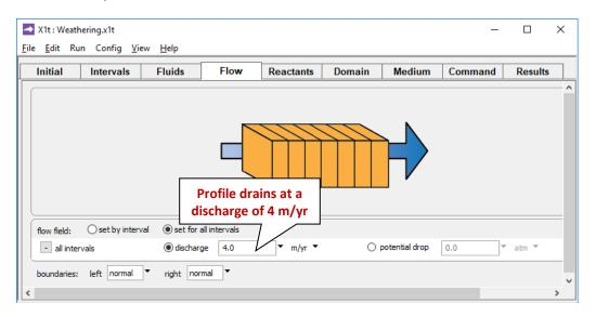
we set up the model to drain at a discharge of 4 m/yr.
