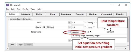
Note that although we've set a heterogeneous initial temperature (as a field variable, using the equation interpreter), we specify that temperature at each point in the domain remain constant in the simulation, assuming in this simple model that conduction away from the fracture plane controls temperature within the fracture. To do so, we clicked the pulldown next to "C" and selected "constant".
