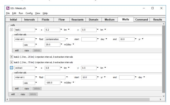
Fluid is withdrawn from the aquifer in the extract well, but none is injected, so no injectate chemistry needs be specified.
