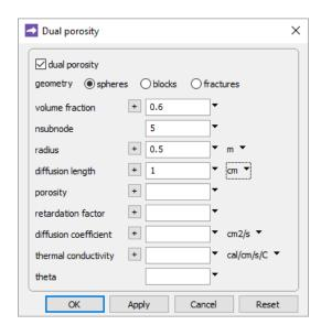
sets the program to consider mass and heat exchange within the outermost 1 cm of the stagnant zones, dividing this length into 10 subnodes. The command
