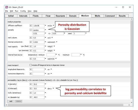
we take advantage of the fact that porosity is carried in the simulation as a field variable by setting it to a random distribution of 35%, with a standard deviation of 5%.
